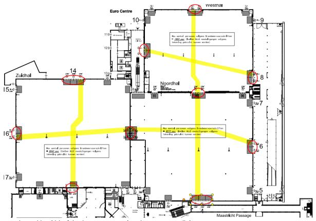
The usable width of the doors must remain at least 5.1 m<sup>1</sup> at all times
